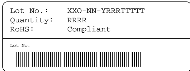
Figure 20: First label on reel: XX = Sensor Type (20 for SHT20), O = Output mode (D = Digital, P = PWM, S = SDM), NN = Chip Version, Y = last digit of year, RRR = number of sensors on reel divided by 10 (200 for 2000 units), TTTTT = Traceability Code.
