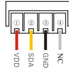
Figure 4 CM2120 Wiring Diagram
