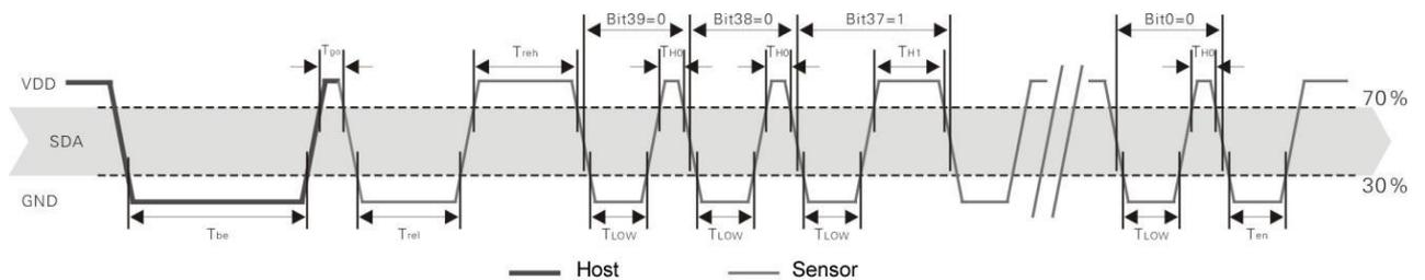
**Figure 7** CM2120 Single bus communication timing
