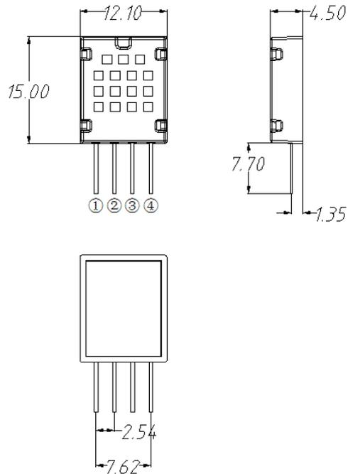
**Figure 1** Dimension (Units: mm)
