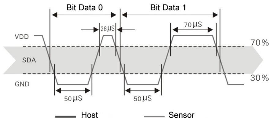
Figure 9 Single Bus Decomposition Sequence Diagram
