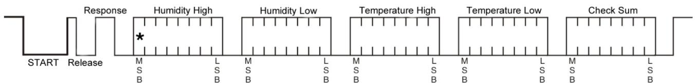
**Figure 6** CM2120 Single Bus Communication Protocol
