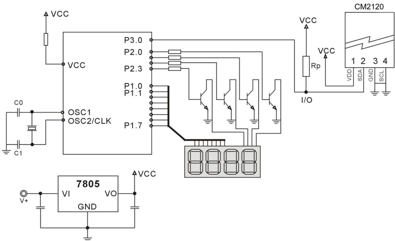
Figure 5 One-Wire Application Circuitry
