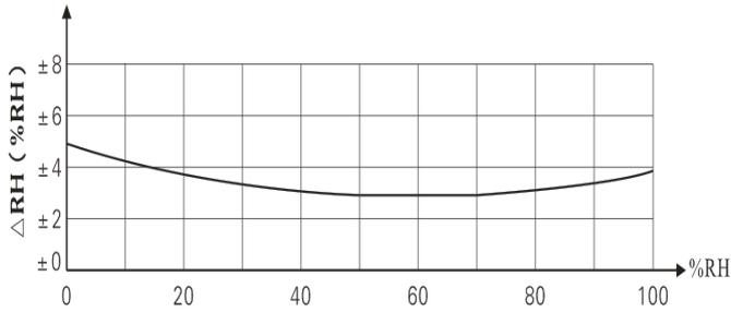
Figure 2 Typical RH% Accuracy at 25°C
