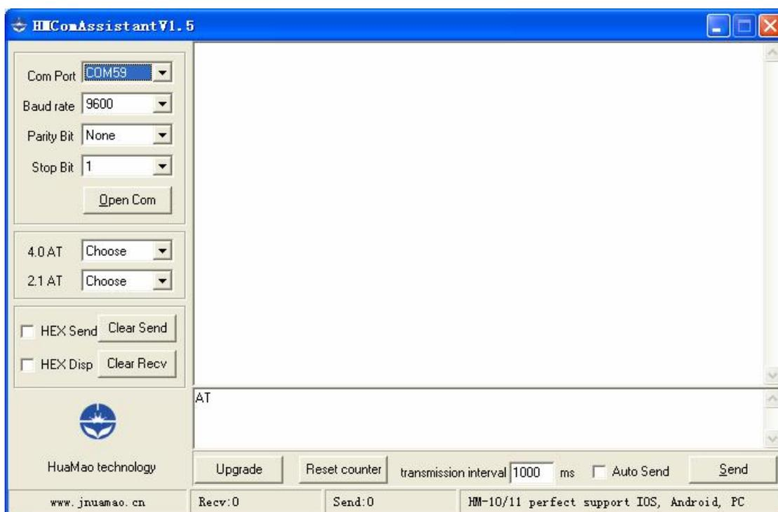
On Transmit version: Only accept AT Command from UART interface when Bluetooth device is not connected with remote device.
