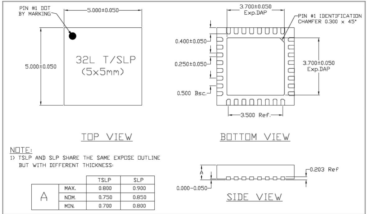
Figure 6-1. ESP8266EX Package
