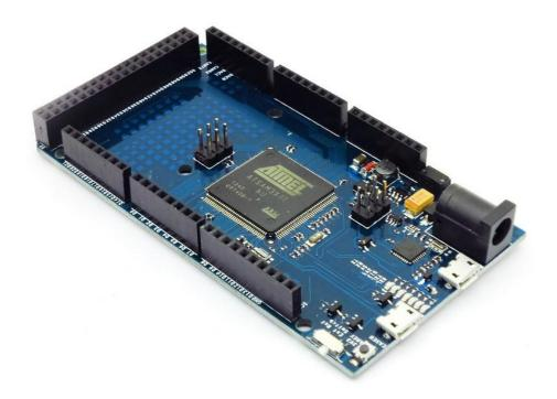
The Iteaduino DUE is a microcontroller board based on the Atmel SAM3X8E ARM Crotex-M3 core. It is the improvement board based on the Arduino DUE. It has 54 digital IO pins, 12 analog inputs, 4 UARTs, a 84MHz clock, an USB OTG capable connection, 2 DACs, 2 IIC, a power jack, an SPI header, a reset button and an erase button.
