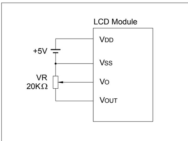
V<sub>O</sub> is LCD driving voltage (contrast adjusting). Adjust V<sub>DD</sub>-V<sub>O</sub> to be around 12.7V for the best contrast.
