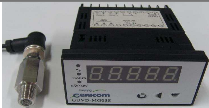
Fig. 1 UV Radiometer 5.0 (Size of Display : 97 × 50 × 112mm)
