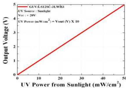
$$\text{UV Power (mW/cm}^2\text{)} = \text{Vout (V)} \times 10$$
