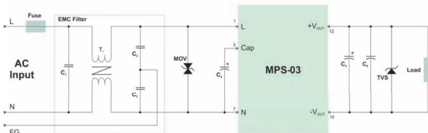
The diagram above illustrates a typical application connection of the MPS-03 series. The top diagram illustrates a DC/DC converter connection while the bottom diagram show the unit connected as an AC/DC power supply. Notes on these circuits are:
