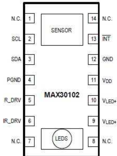
< MAX30102 Pinout ( top view ) >
