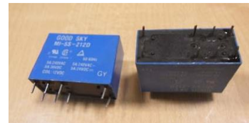
MI-SS-212D. 12V 5A. 8pin. 2 Pole Miniature Power PC Board Relay
