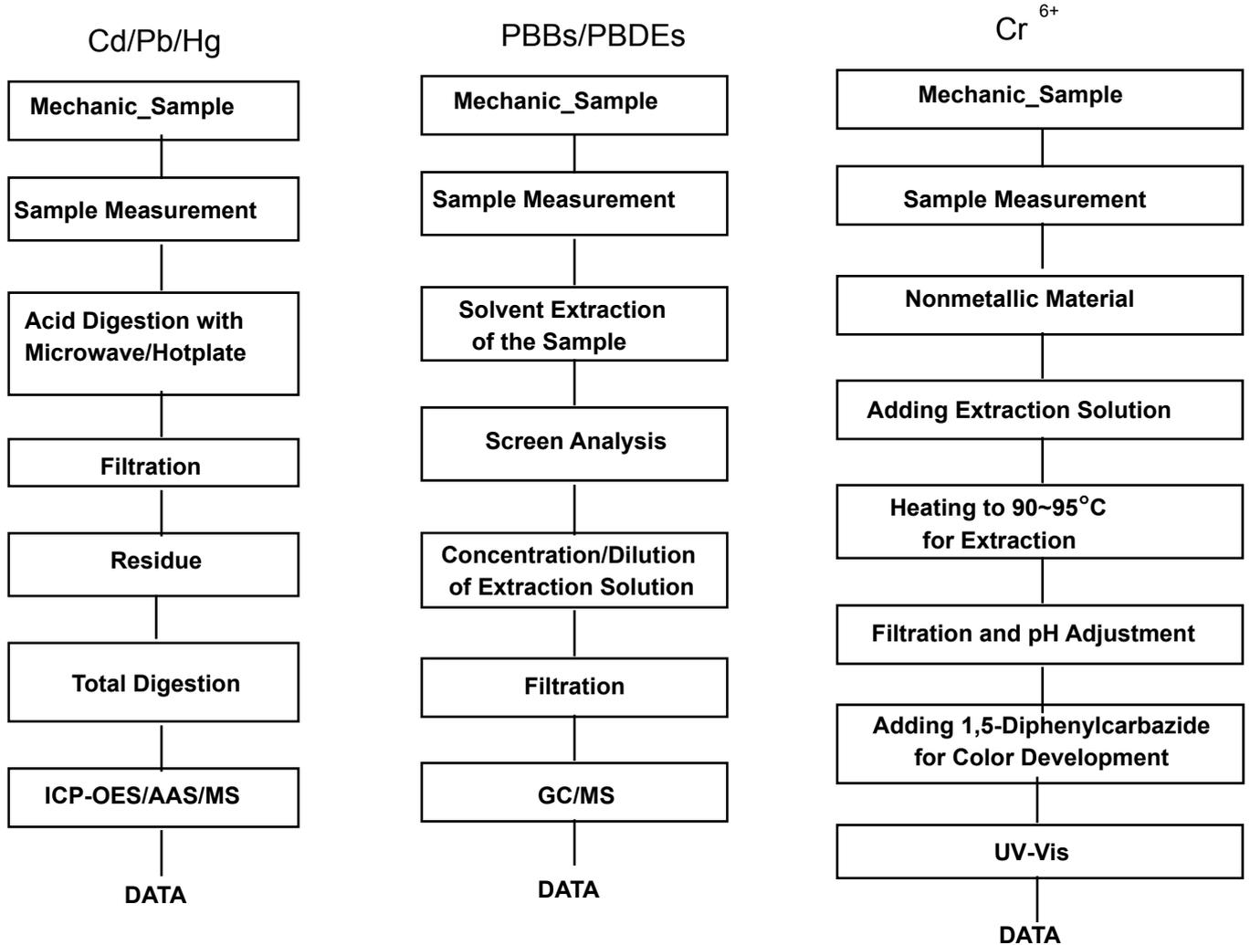
The samples were dissolved totally by pre-conditioning method according to above flow chart for Cd,Pb,Hg.
