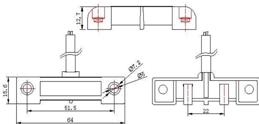
The product utilizes the principle of liquid conductivity for reliable performance and easy installation. When the liquid reaches the two probes of the detector, it sends a switch signal to the alarm host. This product is not used independently. It will not sound an alarm when it meets water.
