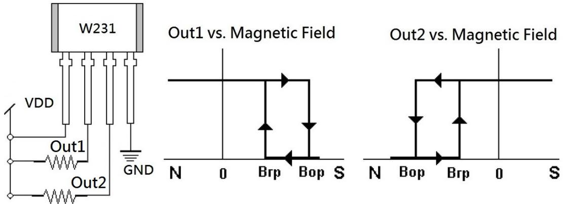
When Out1 and Out2 are short, W231 becomes Omnipolar Hall Effect Switch IC.
