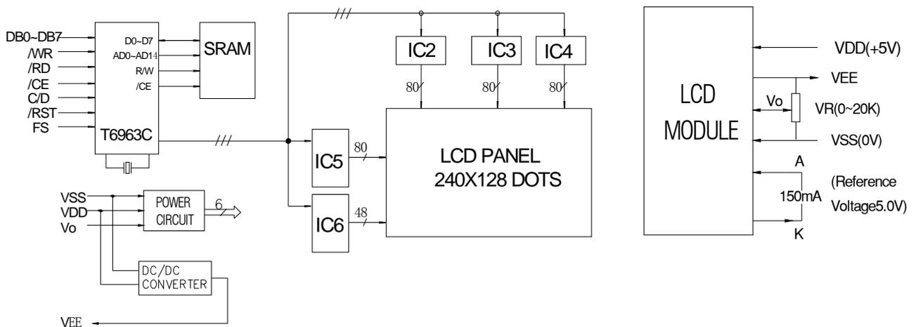
Figure 1. Block Diagram
