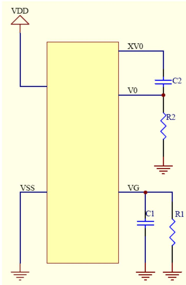
C1=0.1uF~1uF (Non-Polar/6V, default 0.1uF)      C2=0.1uF~1uF (Non-Polar/16V, default 0.1uF)
