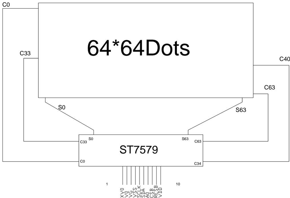
Figure 1. Block diagram
