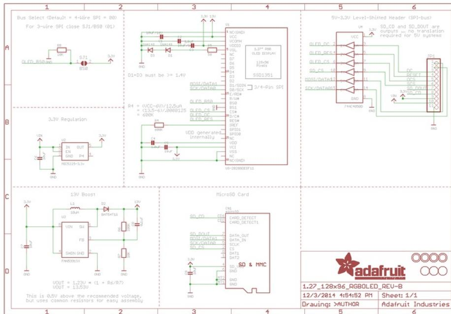
For the level shifter we use the [CD74HC4050 \(https://adafru.it/Boj\)](https://adafru.it/Boj) which has a typical propagation delay of ~10ns
