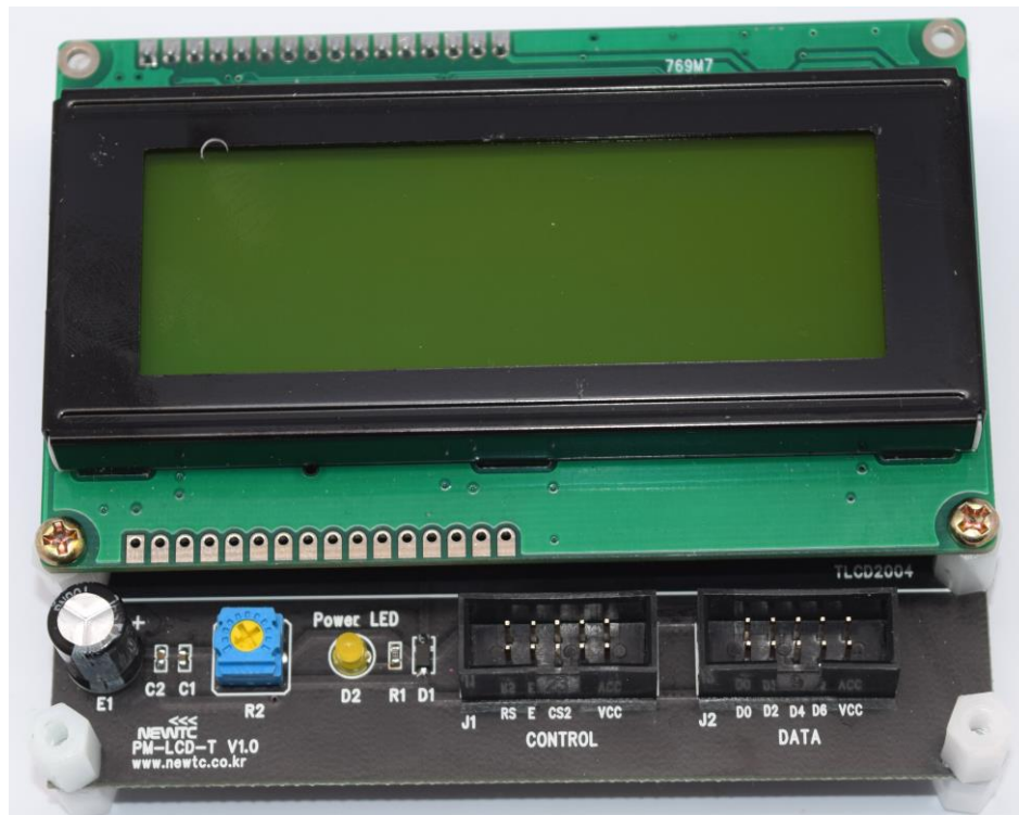
PM-LCD-T 모듈 (PM-LCD-T-420G: 4x20 Text LCD <녹색> 장착됨)
