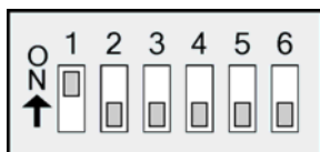
Figure B.8. RS-232 DIP Switch Settings
