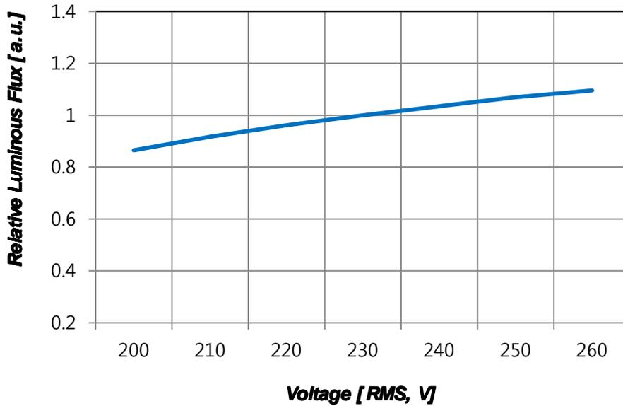
Fig 3-2. Relative Luminous Flux vs. Voltage at  $T_a=25^{\circ}\text{C}$ , 120V
