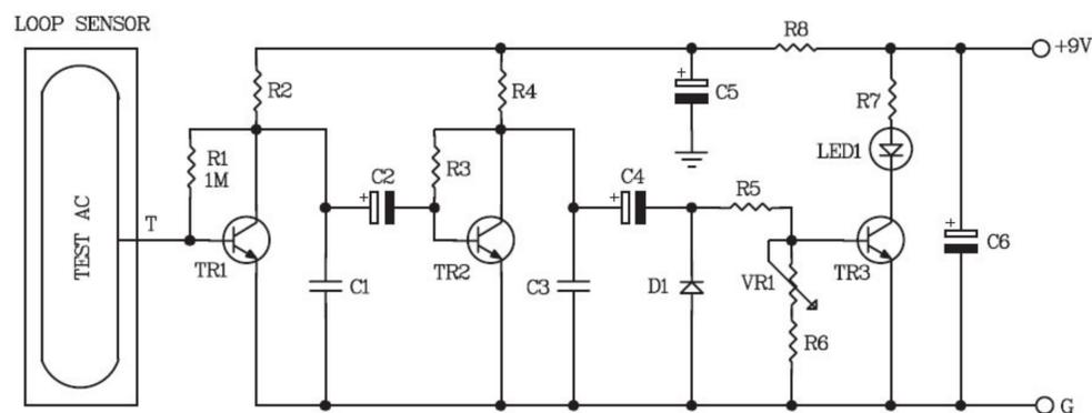
**Figure 1. AC Non-Contact Voltage Detector Circuit**
