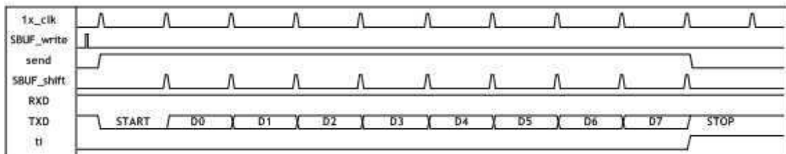
Figure 6.8 Timing Diagram for UART Transmission Mode1
