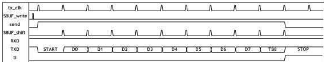
Figure 6.9 Timing Diagram for UART Transmission Mode2
