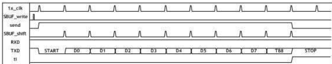
Figure 6.10 Timing Diagram for UART Transmission Mode3
